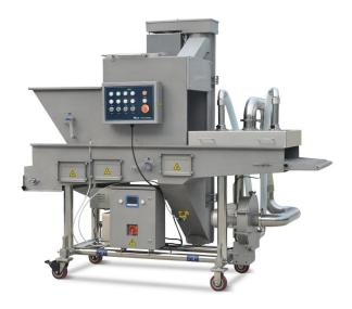
Sprinkle the bread crumbs in the hopper on the mesh belt so that the bread crumbs are evenly coated on the product when the material passes through the mesh belt. It is widely used in chicken, beef, pork, vegetable pie, pumpkin pie and other products.
