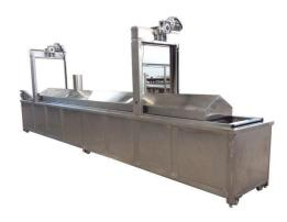
The continuous mesh belt design enables a wide range of applications. The fryer is widely used for frying of various fried foods. And has the function of automatic lifting and scraping.
