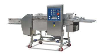
The product is immersed in the slurry so that the product is coated with tempura powder. Suitable for tempura products and sizing products for other fried foods.
